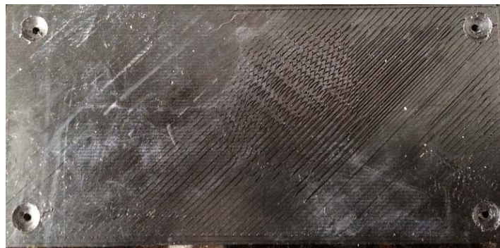
Figure 4.112 – Countersink Holes Complete
