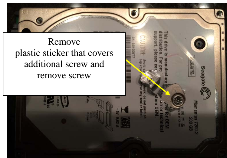
Figure 4.12 – Hidden Torx Screw Removal
